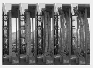
Unreinforced masonry wall under blast load
